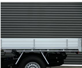
Fully welded & galvanised side coaming
